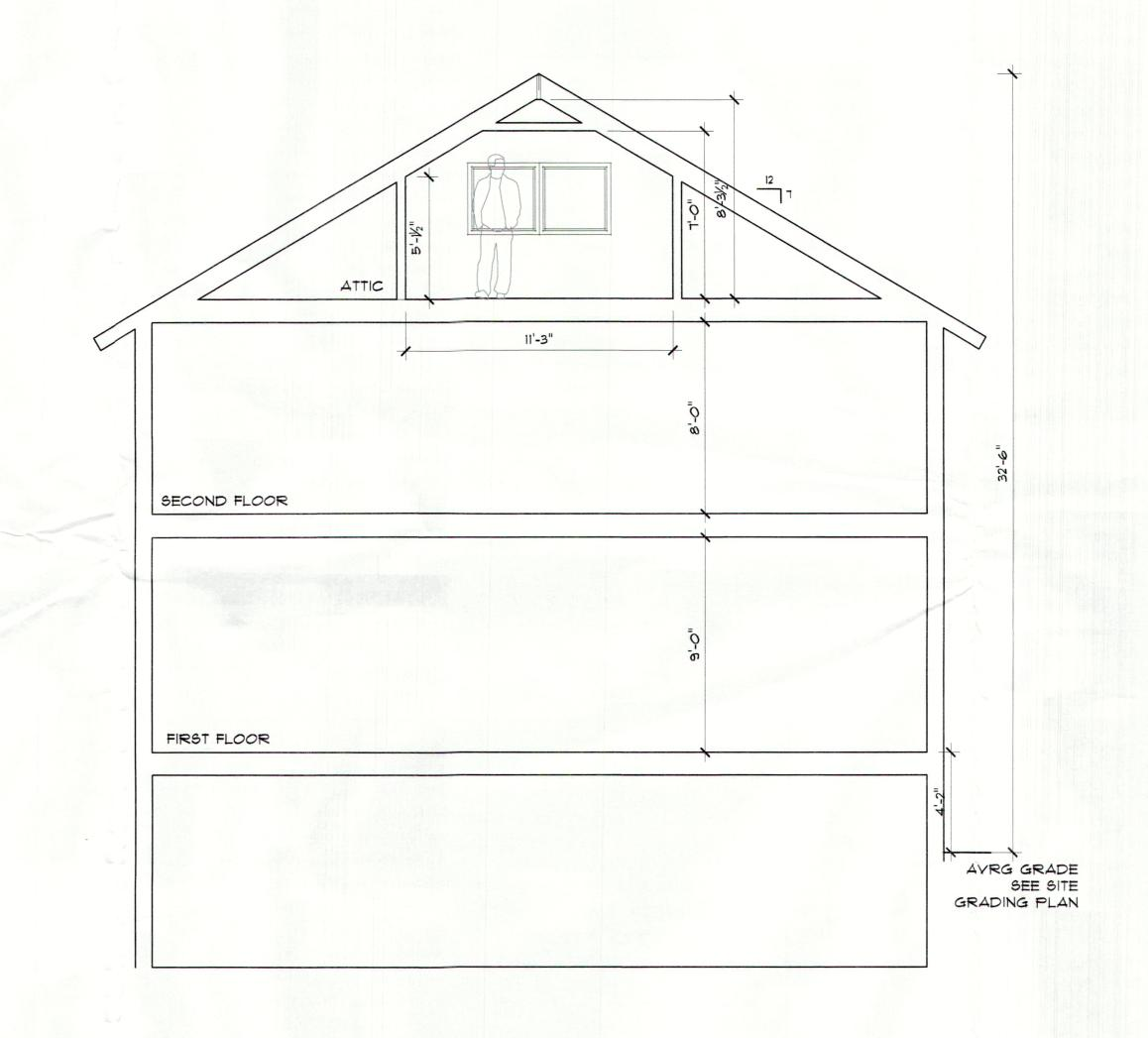
DIAGRAMMATIC SECTION AT 1/12 PITCH SCALE: 1/4"=1'-0"
